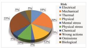
Fig 1. Share of the identified risk factors in electrical installations (UGL - 0.4,-110 kV)
