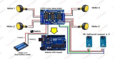
Figure 1: Human Following Robot Circuit
