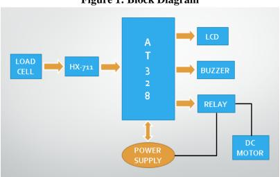
Figure 1: Block Diagram
