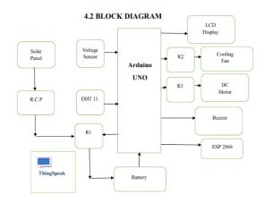
Fig.1 Block diagram of IoT Based Battery Management System
