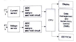
Fig - Functional block diagram of numeric meter
