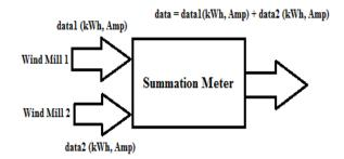
Fig 4 :- Virtual Summation meters for wind mills
