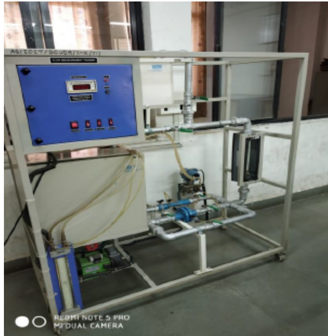
Measurement Flow Level loop
