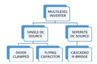
Fig-1: Classification of multilevel inverters
