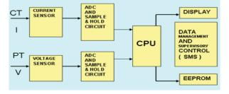
checks various circuits connected to it in a sequential manner. During polling, if some problem is observed with components such as CTs, PTs, battery etc., the meter displays an error message.
