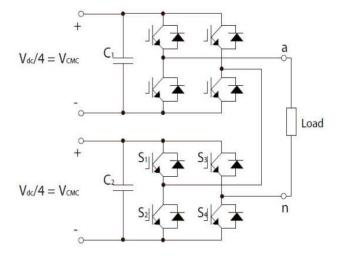
Fig 4: Circuit diagram of cascaded H-Bridge multilevel inverter
