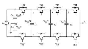
Fig-3: Five-level leg topology of a FCMLI and the output voltage waveform respectively.
