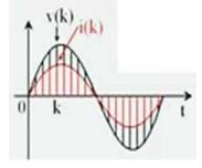
difference between voltage and current is also found out. These values are analogue values. However, the processor of the meter accepts digital signals only. Therefore, the analogue signals are converted to digital form by Analogue to Digital Converter (ADC). The processor processes these input signals to find various parameters such as kVA, kWh, rkVAh and other parameters as shown in following expression.
