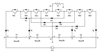
Fig-2: Five-level DCMLI leg topology
