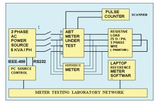
The meter to be tested is connected in series with a standard reference meter. The conditions of full load and unity power factor are generated using the instrument called dimmerstat. The scanner is installed in front of blinking LED of the meter. When one kWh is recorded by the meter, number of blinking pulses recorded by scanner is noted. These are compared with meter specifications and it is decided whether the meter under test is fast, slow or normal.
