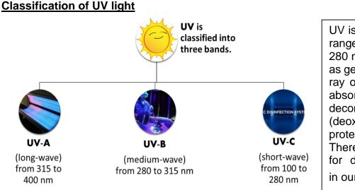
UV is a short wavelength ranges from 100 nm to 280 nm and it also called as germicidal ray. It is the ray of wavelength which absorbs and decomposes DNA (deoxyribonucleic acid), proteins and ozone layer. Therefore, we are using it for disinfection purpose in our project.
