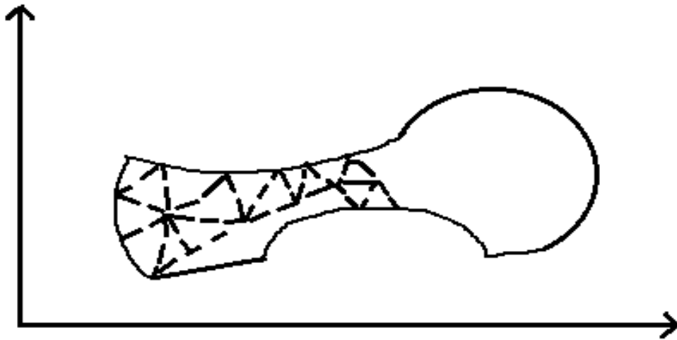
Discretization into triangular elements.
