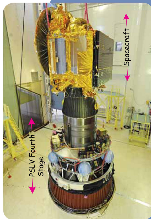
Mars Orbiter Spacecraft mounted on top of PSLV-C25 fourth stage
