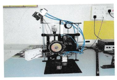
Automatic cutting machine is used to cut metal as it consist of inductive sensor to detect the metal bar and the cutter is adjusted by pneumatic cylinder which is controlled by throttle valve.
