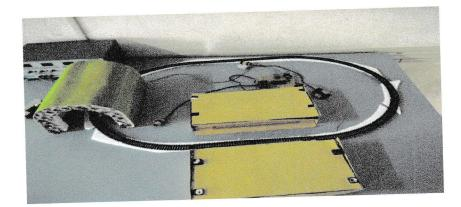
This project is about automatic platform joining system for locomotive of public .In this we used two ir sensor to detedt train and on detection of train the platform opens and on departure of train the platform joins together.
