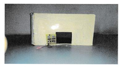
It is counter which is used for detecting object while dispatching so that the count of product can be done. It have a ir sensor which gives signal to counter ic and the counts are displayed on 7 segment display.
