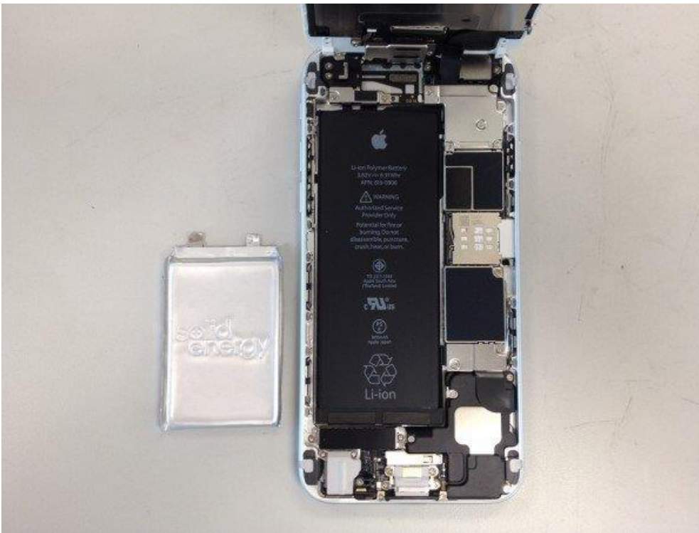
The lithium-metal battery compared to a lithium-ion battery seated in an iPhone. Image courtesy of Business Wire.
